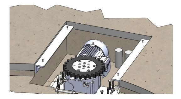
6. Position drive motor inside pit for anchoring in step 9.
