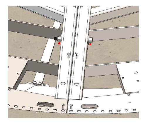
10. At this time, before installing top panels, get motor assembly positioned with urethane pinion gear teeth meshed with drive pins on turntable. Set motor assembly where there is 1/8" of spacing/backlash between pinion gear teeth and drive pins and anchor motor down with (4) concrete wedge anchors in holes shown below. The motor backlash is also adjustable using jack screw and lock down nuts on motor mount plate.
