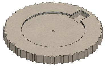
Position slew bearing in the center point of the turntable pit and anchor in place with (3) 3/8" x 3.75" concrete wedge anchors marked with red dots below. Cut off exposed threads above nut (if any) to allow clearance of paneling above.
