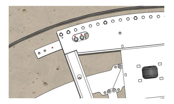
8. Repeat step 5 with consecutively numbered pie sections in a counterclockwise direction. Be sure to leave all hardware loosely fastened.
