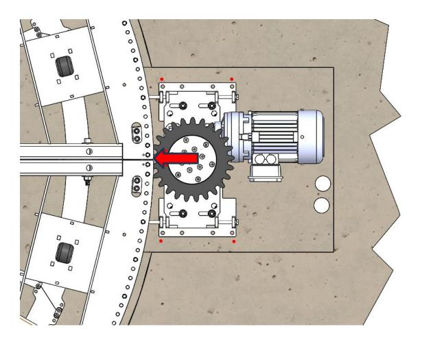
11. Layout panels starting with the center panel then panel #1 attaching to pie section #1 and loosely installing M6x16mm FHCS and moving in a counterclockwise pattern until all twenty panels are positioned in place. Tighten screws once all panels have been positioned in place.
