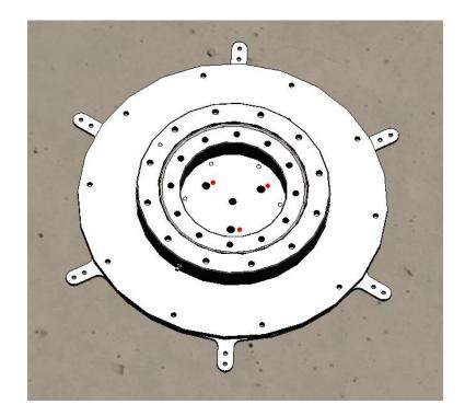
3. Layout wheel track sections along with alignment spokes and fasten everything together with M8x12mm BHCS and M8 Lock Washers.
