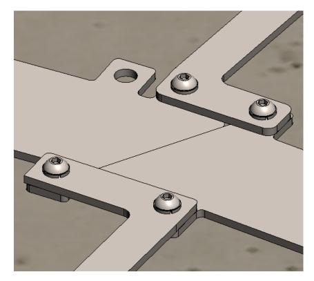
5. Install/Anchor hatch support angles to the walls of the motor pit using supplied concrete wedge anchors. Anchor the angle support 3/16-1/4" below the finished floor (depending on top surface option) and parallel so that the hatch panel sits flush once installed.
