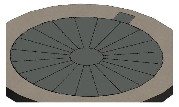
12. Install hatch panel using a drill to match drill and tap holes in angle in place for a best fit to turntable edge. Use M6x16mm FHCS to fasten and the installation is completed.
