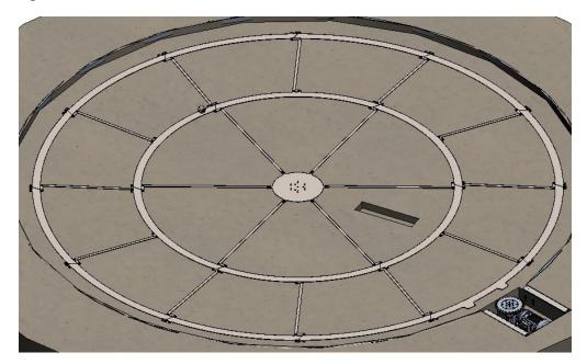
4. Once all track screws have been tightened. Install a concrete wedge anchor at each track joint and cut off remaining threads above nut to allow clearance of tube structure. Then apply the supplied grease to the track to lubricate the wheel contact area.
