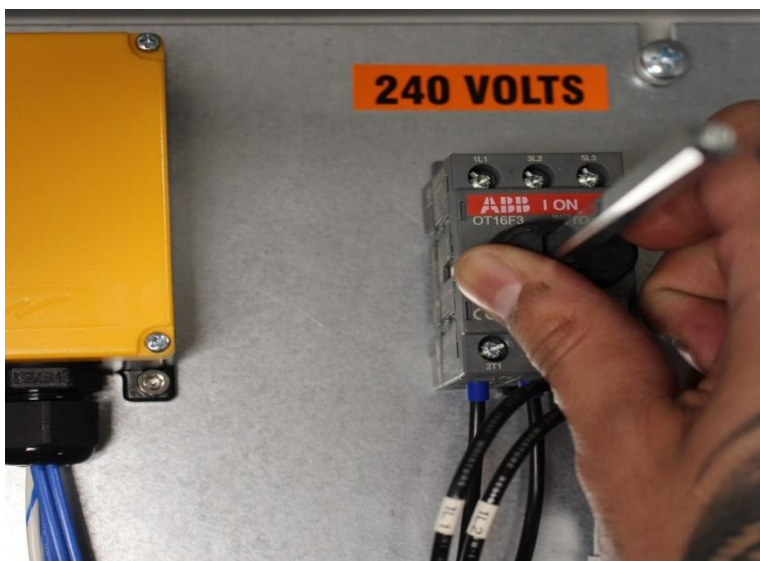
Manually turn power supply on inside control box.
