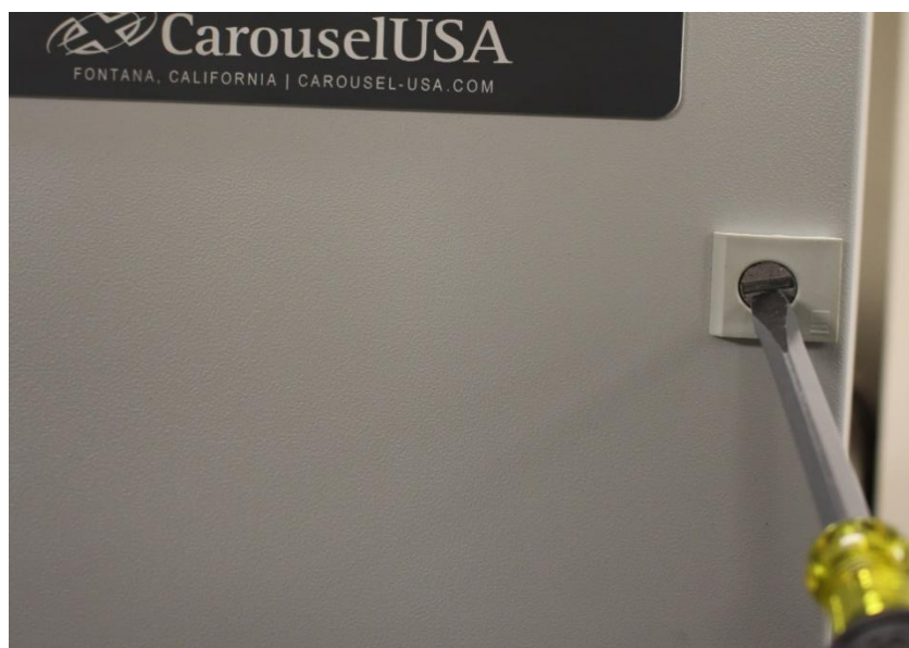
Open control panel using coin, key, or screwdriver.
