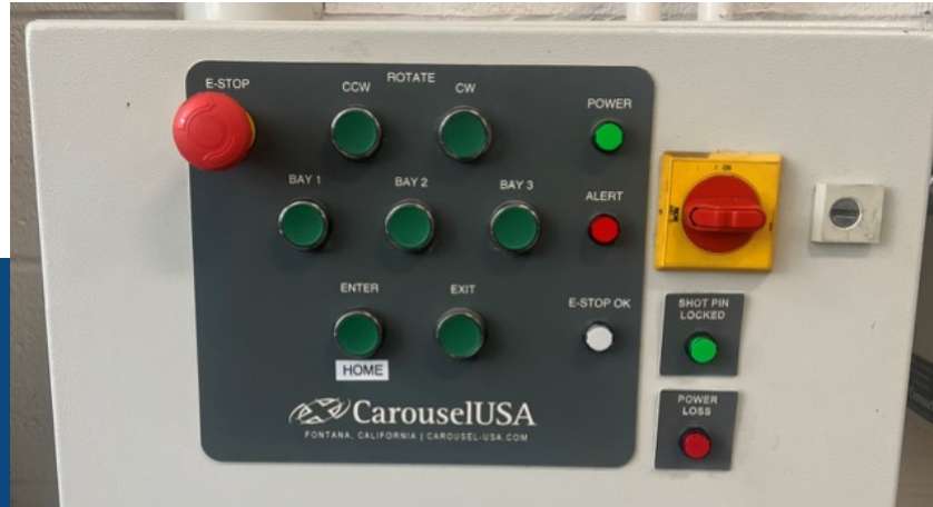
Figure 2: Control panel door operators with added shot pin locked and power loss indicator lights.
