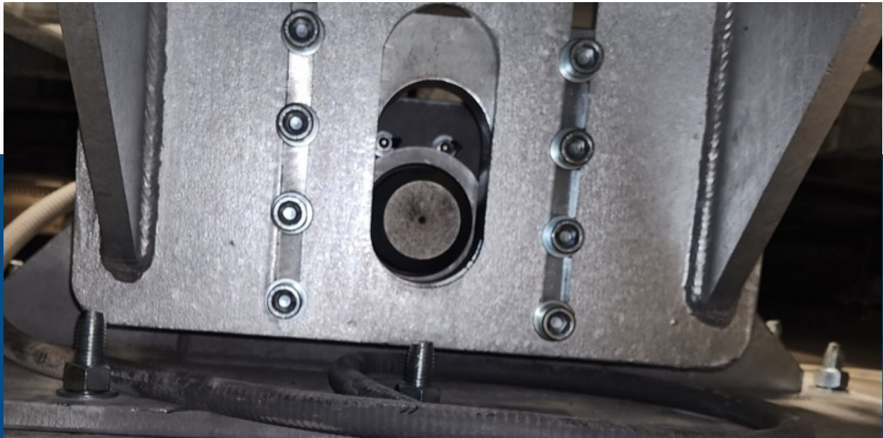
Figure 1: Shot pin aligned with receiver, underneath the top surface of the turntable.
