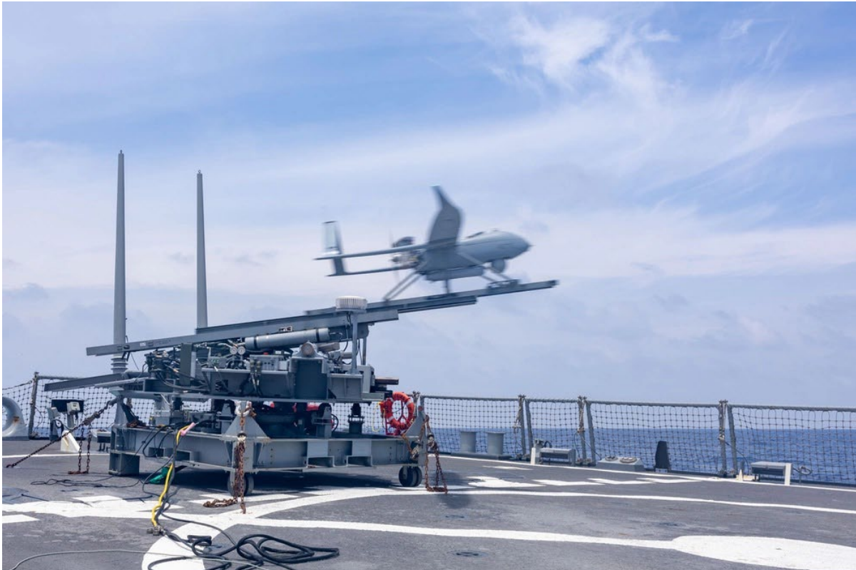
Aerosonde UAS launching from the L&R system aboard a U.S. Navy ship
