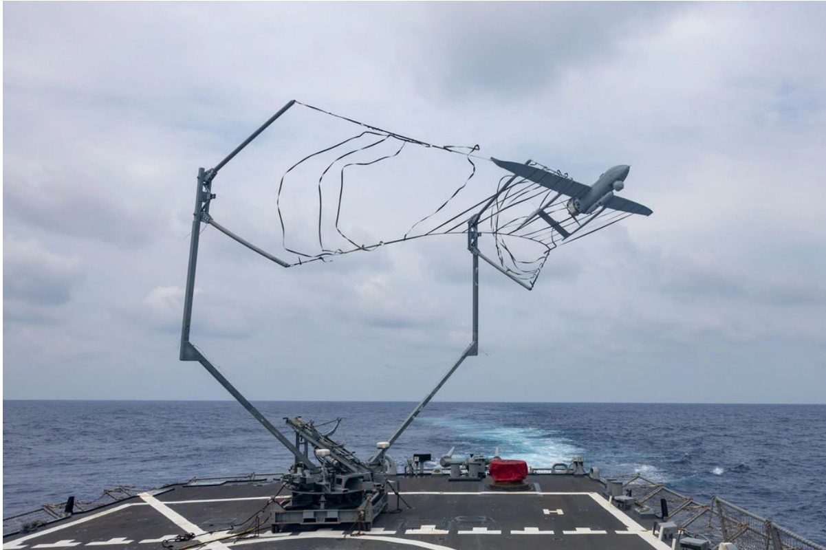
Aerosonde UAS approaching the Launch & Recovery system aboard a U.S. Navy vessel
