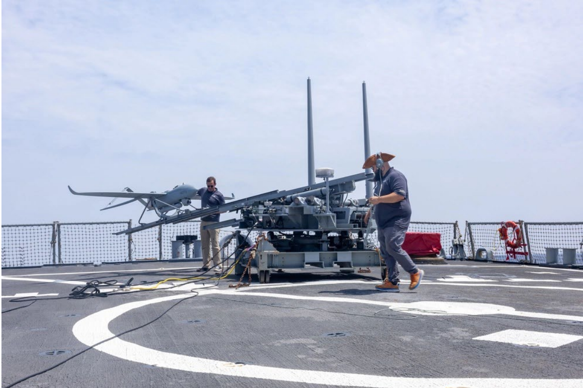
The Aerosonde L&R system in operation aboard a U.S. Navy ship — the Carousel-USA turntable rotates the entire assembly to face into the wind
