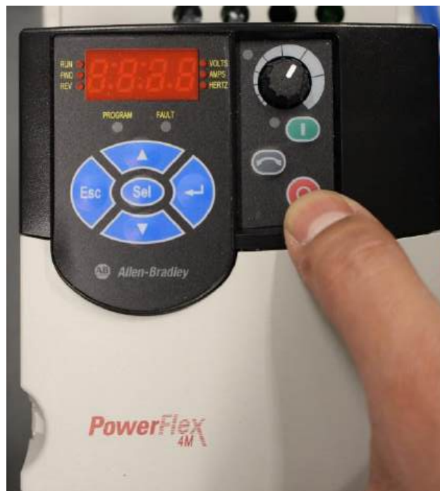
VFD Fault Reset Button
