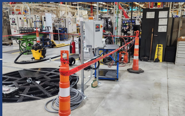
The completed 24SRI turntable — smooth steel top with flush-mounted tracks (left), and the tubular steel structure set into the pit alongside the Carousel-USA control panel (right).
